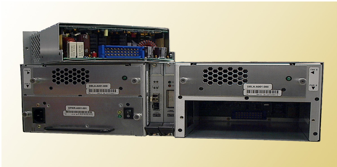
Exhibit 7-4: A power supply pulled out from a rackmount Diamond Storage Array: do not leave an empty opening while the Diamond Storage Array is operating. Access the blower assembly and the power supply by loosening the screws on either side of the component, then pulling out the part. If a blower or power supply stops working, keep it in place until another component is installed. (Note: host interface configuration pictured is not supported)
